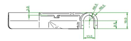
The pipe bend support **stabilizes and protects** the pipe at the bending point.
